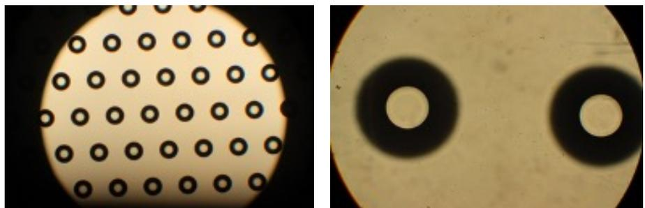
**Figure 3a:** Examples of holes designed for optical fiber in a borosilicate glass after 96hrs of HAST, (a) low magnification and (b) high magnification.
